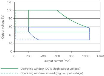
Operating window 100 % (low output voltage) Operating window dimmed (low output voltage) Make sure that the LED Driver is operated within the given window under all operating conditions. Special attention needs to be paid at dimming and DC emergency operation as the forward voltage of the connected LED modules varies with the dimming level, due to the implemented amplitude dimming technology. Coming below the specified minimum output voltage of the LED Driver may cause the device to shut-down.
